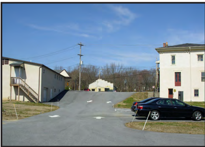
Extra wide curb cuts are not pedestrian-friendly, as they interrupt sidewalk activity.
