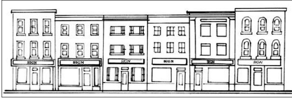
FIGURE SD-3 Sign Placement
