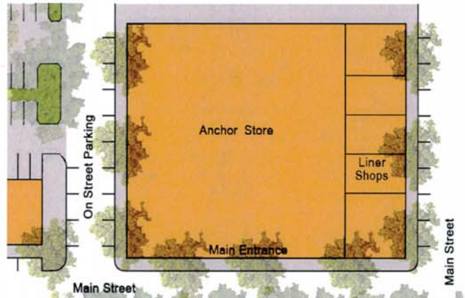
Lot Diagram: Anchor store with liner shops maintain the established Build-to Line.
