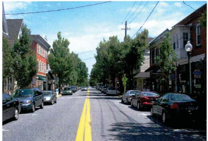
On-street parking buffers pedestrians on Main Street (Litz, PA)
