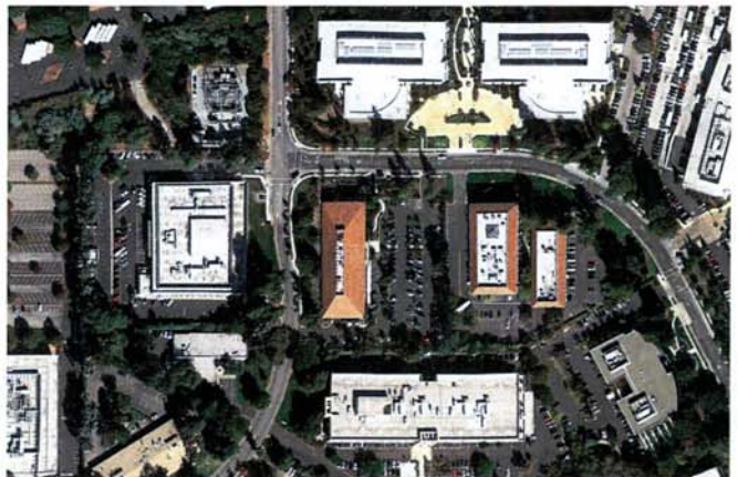
Stanford Research Park, Palo Alto, CA: Industrial and technology campus with buildings lining the streetscape, parking to the side and rear, and central plaza space.
