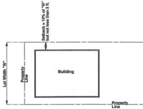
10.40.080-A NARROW PARCEL SITE PLAN: Building Setbacks for Narrow Parcels (Less than 50 ft.)
