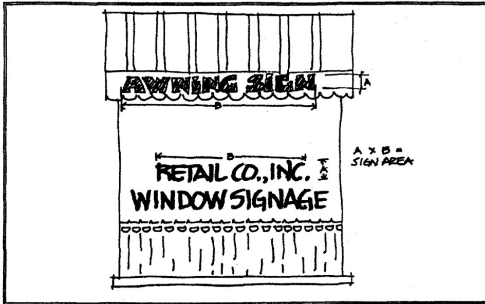
SIGN ILLUSTRATIONS: AWNING AND WINDOW SIGNS
