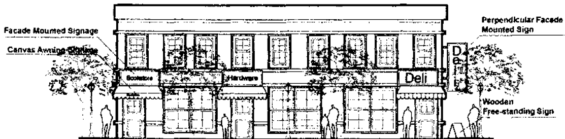
Figure F. Signage.
