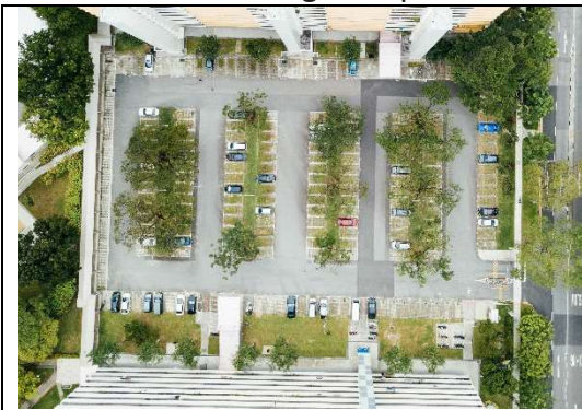
Parking lot with perimeter landscaping, landscaped islands, and shared parking between two commercial uses to minimize curb cuts.
