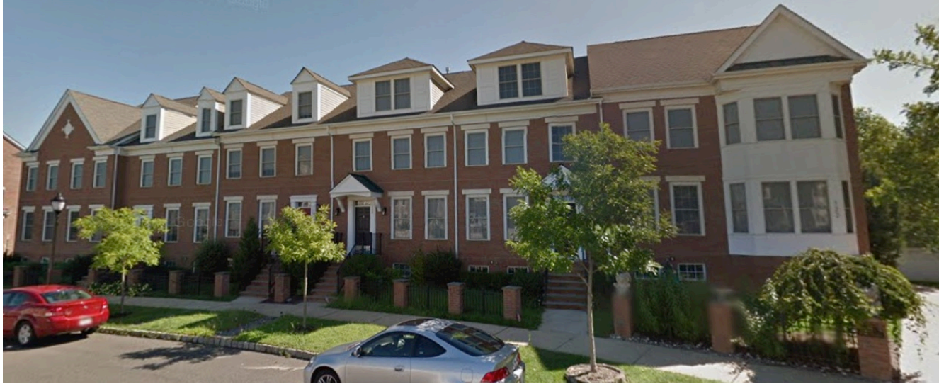
Townhouse building type with appropriate architectural style in Robbinsville, NJ. Parking is located behind the building. Access to each dwelling is via a stoop, and a fence with piers demarcates the boundary between the public and private “realm”. Street trees, a generous grassy verge, and sidewalks are attractive streetscape elements.
