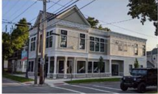
Figure 15. This new building exemplifies many desired design elements including facade breaks, use of traditional windows, short setbacks to the street, and traditional siding. This building could house commercial on the ground floor, and commercial and/or residential on the second floor.
