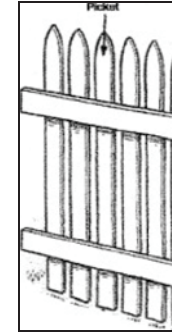
Figure 14: Typical picket fence detail
