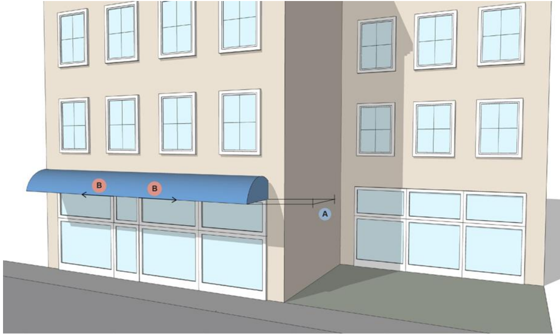
Figure 225-20-B: Front façade recessing
