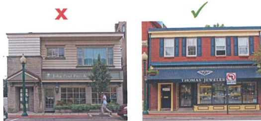
These local buildings are very similar in massing, but use different compositional strategies. The right image demonstrates preferred glazing styles, fenestration patterns, finish materials and colors, and facade detailing.
