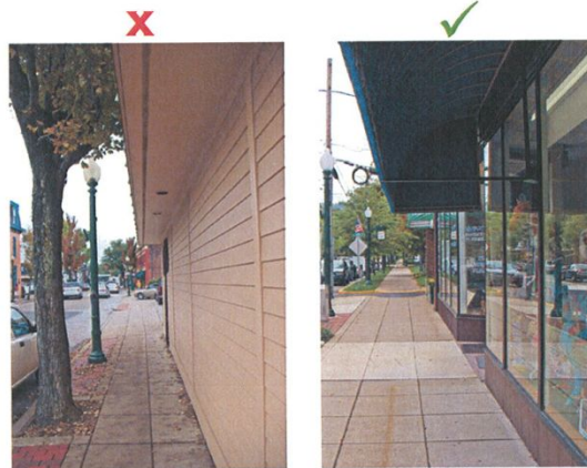
Two local storefronts demonstrate the difference that facade transparency makes from the pedestrian's perspective.
