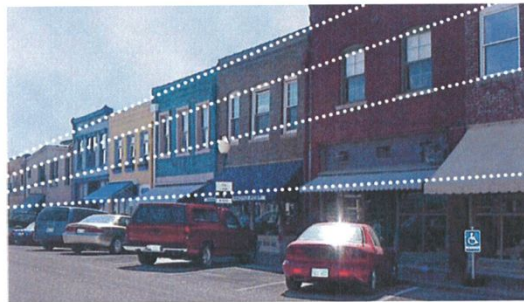
A similar village main street shows how similarities in the location of facades, windows, doors, cornices and other elements help define character.
