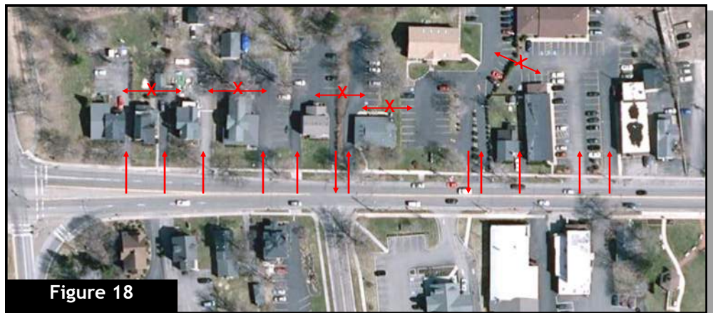
The arrows highlight the issues associated with individual access points and a lack of cross access between properties along primary roadways. The numerous turning movements reduces transportation safety, while the constant break in the street line hinders the rhythm of the streetscape and degrades the pedestrian experience.
