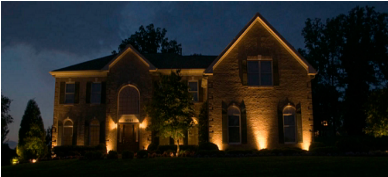
Figure 9-18-7 Example of Poor Up Lighting
