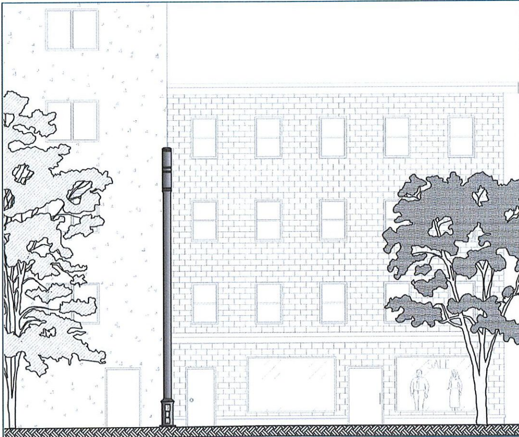
Freestanding Small Cell Facility located in commercial area
