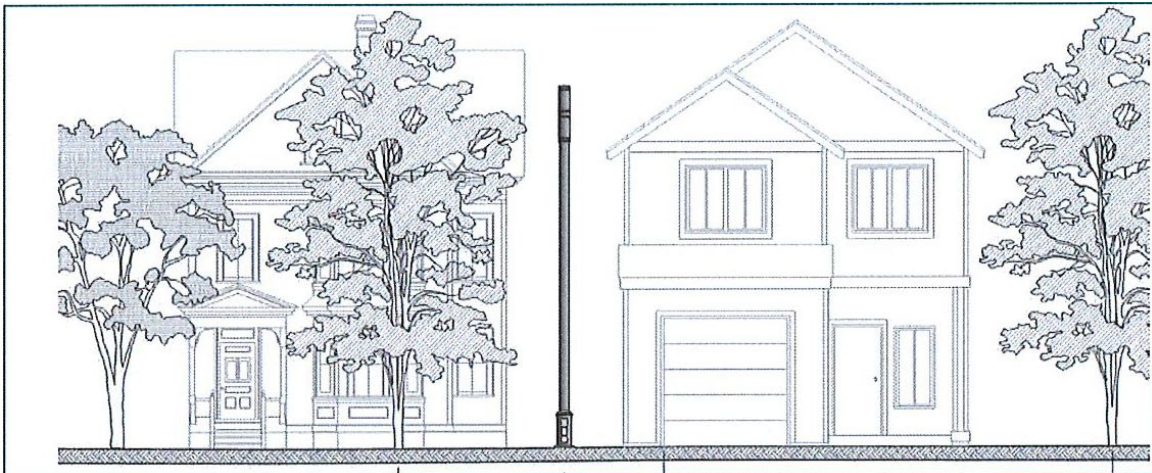
Freestanding Small Cell Facility located between property lines and trees
