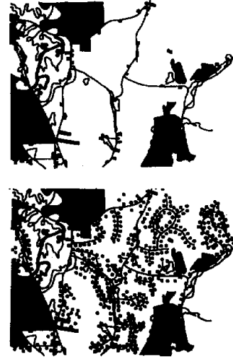
Figure 2 A matching pair of graphics, taken from an actual "build-out map," showing existing conditions (mostly undeveloped land) contrasted with the potential development pattern of "checkerboard suburbia" created through conventional zoning and subdivision regulations.
